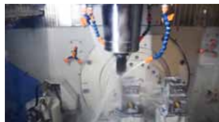
➤ Simultaneous 5-axis machining center DVF 5000 performing thread cutting operations.
